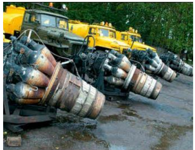
Example of forced heat Transfer Heavy Snow Removal Equipment
