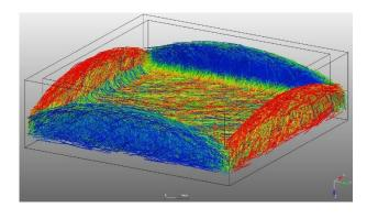
Figure 2: Flow and fiber orientation simulation in 3DTimon
