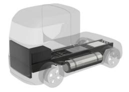
Figure 2: Hydrogen-powered truck concept [Cryomotive]
