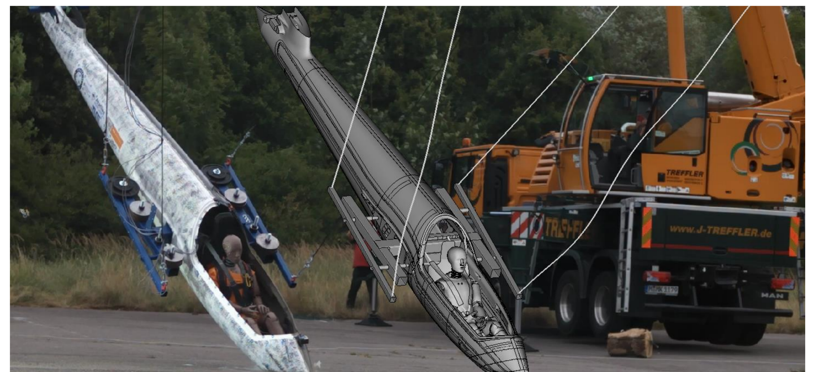
Fig. 3: Sailplane crash test and simulation [Thesis Hofmann 2022]
