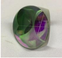
d retroreflector with added optical filter layer. Layer is optimized for transmission of 532 nm. Reflector diameter is approx. 38 mm.
